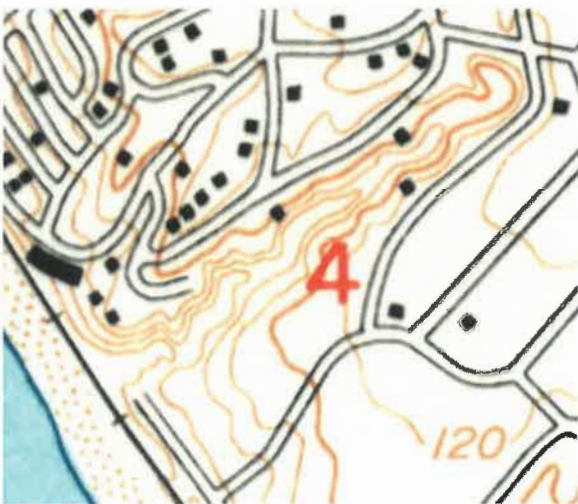
Figure 4. Topographic map from 1948 showing Trafalgar Canyon. Narrowing of the canyon near the mouth is visible in the topographic lines.
